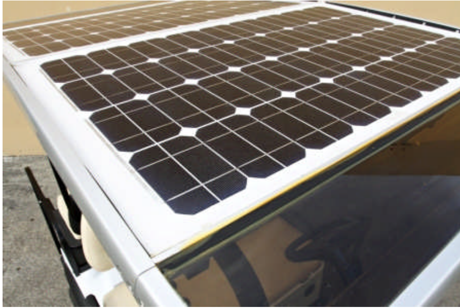
SOLAR DRIVE 200 WATT TOP ON EVERGREEN VEHICLE
